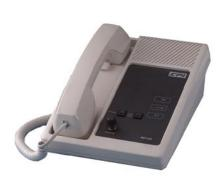
The RST300/PST300 remote system allows fixed site users access to the transmit and receive functions of the G2 unit from any 2 wire voice grade pair. This allows in building operation away from the main G2 unit and in areas where antenna placement may be a problem. All parallel remotes receive all incoming and outgoing audio as well as provide LED indicators of the G2 status indicators.
