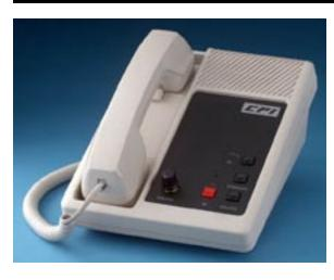
The DR series DC remote control units are designed to provide control of a remotely located base station over an in-house or leased metallic wire pair. The DR series units use a simple dip switch to select the desired control current and other features. Standard features include: receive and transmit audio compression, front panel transmit capability, line continuity sensor, parallel cross mute, line operated PTT indicator, and 2 watt audio output.
