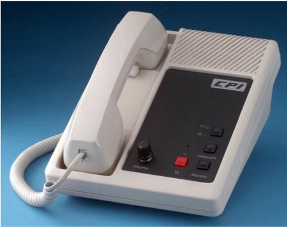
The TR series tone remote control units are designed to provide control of a remotely located base station or repeater over a voice grade wire pair. The TR series units use the EIA standard sequential tone format which provides 2175 Hz. guard tone, 1950/1850 Hz function tones, 2050 Hz. monitor and 2175 Hz. hold tone. Standard features include: receive and transmit audio compression, front panel transmit, PTT indicator, and 2 watt audio output.
